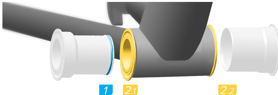
Use a headset press or bottom bracket bearing press tool to install the drive side bearing cup into the frame according to the tool manufacturer's instructions. Repeat the installation with the non-drive side bearing cup.
