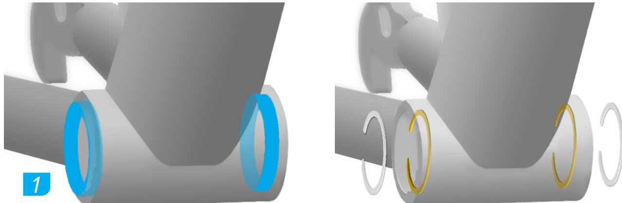
**2** **Frames with retaining ring grooves only:** use a flat blade screwdriver to seat the circlips into the grooves.
