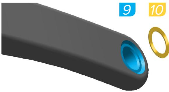
Install a washer between the crank arm and pedal. Tighten the pedal shaft to 47-54 N·m (416-478 in-lb).
