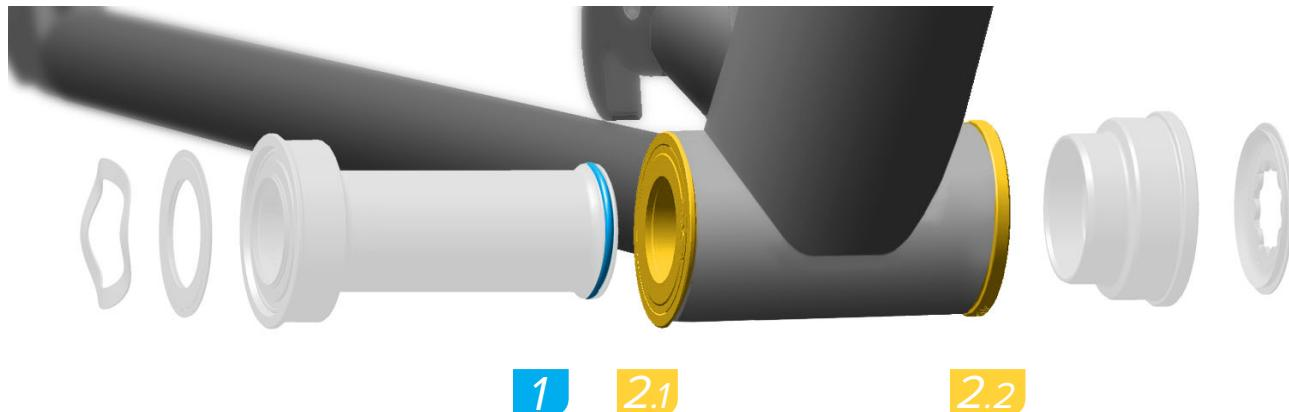
Use a headset press or bottom bracket bearing press tool to install the drive side bearing cup into the frame according to the tool manufacturer's instructions. Repeat the installation with the non-drive side bearing cup.
