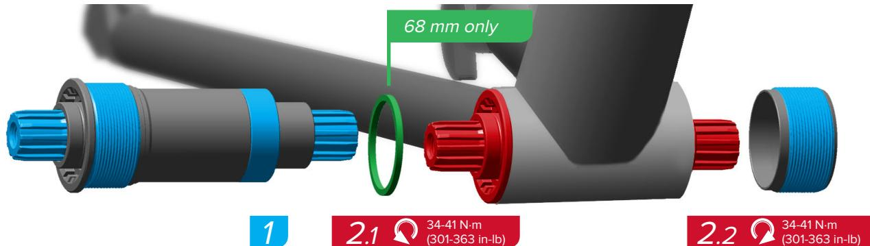
Use a Power Spline bottom bracket tool to tighten the drive side cup to 34-41 N·m (301-363 in-lb). Use a Power Spline bottom bracket tool to tighten the non-drive side cup to 34-41 N·m (301-363 in-lb).
