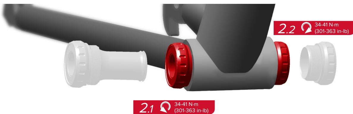
Use a GXP bottom bracket tool to tighten the cups into the frames.
