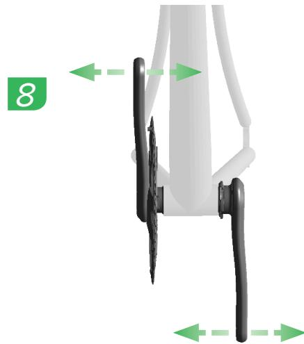
To preload the crankset, turn the preload adjuster in the direction of the + sign until it stops. Tighten the preload adjuster bolt to close the gap. Check the crankset for play by rocking the crank arms back and forth.
