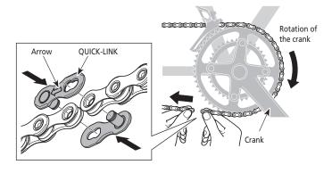
2. Use Shimano original tool TL-CN10 to slide the pins and insert them firmly.
